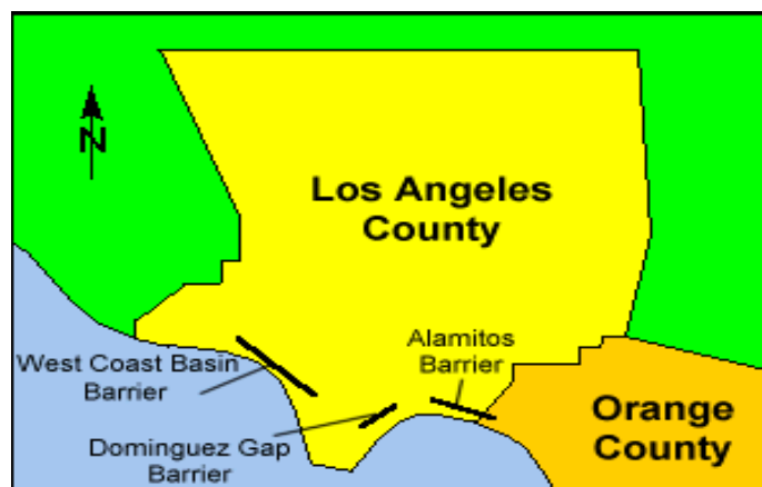
Figure C-3 7 Los Angeles County Seawater Barrier Projects
